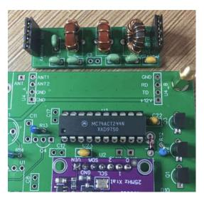
Plug the pin header sockets to the main board and solder.
