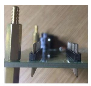
Plug in the Nano module. Make sure the USB port is at the main board edge. Watch out the holes in the four corners. Solder all 30 pins.
