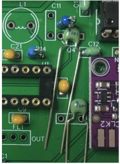
The photo shows the center pin of Q4-BS170 to make sure it is safe from static.
