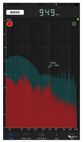
If you have access to the tinySA, you can use the signal generator function to inject 28075kHz, -85dBm together with a fixed attenuator (-30 or -40dB) in between, and monitor the receiver spectrum of ADX-S with WSJT-x or JTDX. Do the calibration at power up, until you see spectrum like this.
