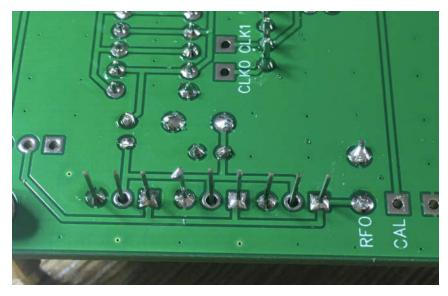
Make sure your solder iron is well grounded. If not, you can unplug the power of your solder iron and solder the 3 center leads.
