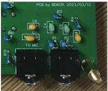
Use an audio signal generator like Sonic Tools App on iPhone to inject audio to CON1-TO SPK jack. Turn the volume to MAX and it should trigger TX, and the TX LED should be on. When you perform this test, please make sure the 50 ohm load is still connected to J1-BNC.
