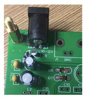
Now let's do a test to make sure the 12V does exist on VIN pin of XA1 – Arduino Nano module. Use the DVM for voltage measurement of about 12V. The red probe goes to the VIN pad, while the black probe goes to ground pad of the BNC connector. Plug in the 12V power supply (center positive) and measure. Looks good so far.
