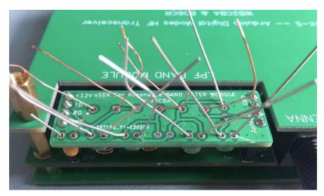
Use a marker pen or label to mark the LPF band filter board.
