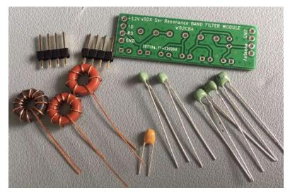
It is recommended you use the sockets on the main board as support. Populate the parts correctly and solder. Always remember, C7-100nF is near to the black toroid, and the red toroid with more turns is in the middle of 3 toroids. Some schematic and BOM of the original design ADX does not match the PCB very well, so please double check the ADX-S BOM.
