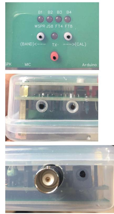
You can mark the USB port location with a short line, drill two holes, enlarge them and join them. The finished chassis looks like this.
