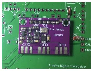
Turn the main board and solder the pin headers. Again, don't need to trim the extra leads.
