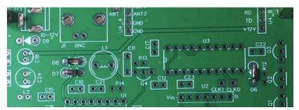
Bend the leads so they will not drop after you turn the PCB for soldering. If your soldering station supports temperature adjustment, you can adjust to 350C. It is good for both the leaded or lead-free solder wire. Solder about 3 seconds for each pad. Don't solder too long time.
