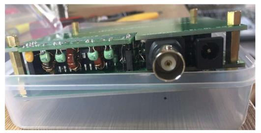
Drill a small hole, enlarge it gradually so you can protrude the BNC connector. The electric drill sold by IKEA for screw fastening will do the job here.
