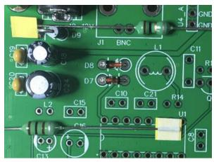
Solder L2, C13-10uF, C1, C16-100uF, C2, C14, C15-100nF. Beware of the polarity of C1, C13 and C16.
