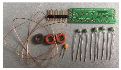
Wind the toroids based on the BOM, and prepare the pin headers and capacitor leads. The black toroid has 12 turns, and the red toroids have 10 turns and 7 turns. Remove the enamels of the wires ends before soldering. Some people use sandpapers. Wire length: 1.5 cm per turn plus 5 cm. For 12 turns, the length is 23 cm.
