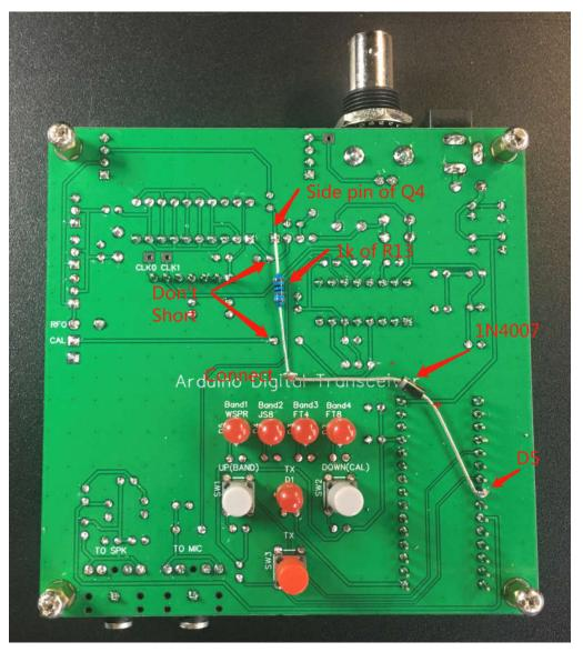
The 1k resistor is originally used for R13. Once you press both UP and DOWN buttons, the firmware will toggle D5 pin and it will act as a switch for ATT.
