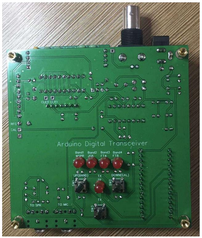
Now you can put on the top cover and fasten the screws. Put on the caps of the switches. Red for SW3-TX.
