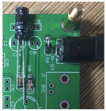
Likewise for C24 – 100uF. Solder C18, C19-100nF, C20-100nF, and C24.
