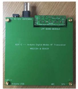
Check out the stack of the sandwich and the standoffs to make sure they are right. If you identify the risks of potential short circuit, please correct them before you apply power supply.
