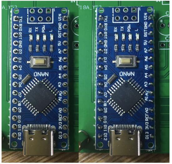
Turn the main board and solder all the leads of the pin headers. Don't need to trim the extra leads.
