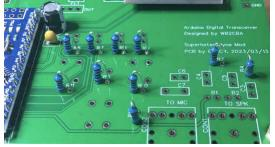
The long lead of the red LED goes to the + marking pad of D1.
