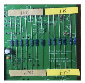
Populate R16, R17-10K as close to the PCB as possible and solder. The 5351 module has a 8-pin header but it only needs 7 pins, so you will need to trim 1 pin first, and plug in the 7-pin header, again, shorter lead side on the top.
