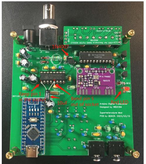
The red LED will reduce the amplitude of CLK2 (BFO) and also indicate the existence of CLK2 (BFO). The 10uF will enable AGC of CD2003. The 1N4007 in place of R13 is used as an attenuator in the RX front end.
