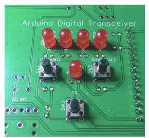
Now press and hold the SW2-DOWN(CAL) button and plug the power supply until you see both B1 and B4 LEDs are on. Now you can probe on the test point CAL using a frequency counter or other test instruments like an oscilloscope to see if you can get a 1MHz square wave. Please note,
