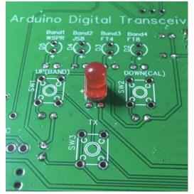
Populate D2-D5 and SW1-SW3 as close to the PCB as possible and solder.
