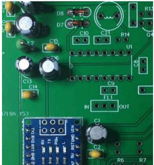
You can plug in the 12V power supply (center positive) again and test on pin 15 of U1-CD2003 to make sure the +5V power supply for CD2003 exist.
